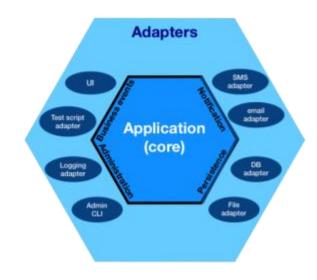
Figure 5: Hexagonal architecture pattern [19]
