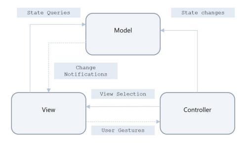
Figure 4: Original MVC architecture pattern [20]
