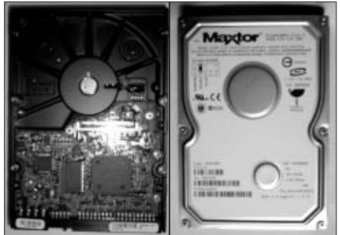
Figure 22 – The back and front of a Maxtor-DiamondMax Plus 9 ATA-133 80GB 7200 rpm Hard Drive
