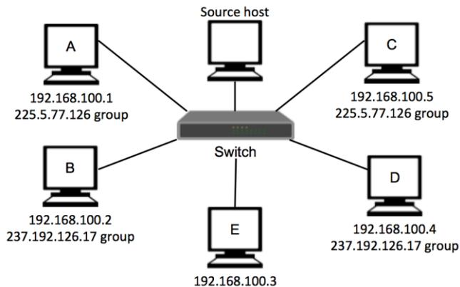
Identify which devices will receive the packet if the destination IP address and the type of IP address each is (unicast, broadcast or multicast).
