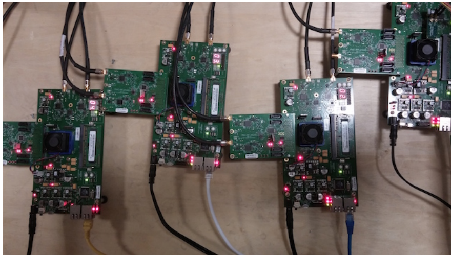
Figure 4.13: Each AP is a latest WARP v3 Kit with FMC-RF-2X245 module to enable four radios. Antennas are placed at the dedicated AP positions with low loss LMR-400 cables.
