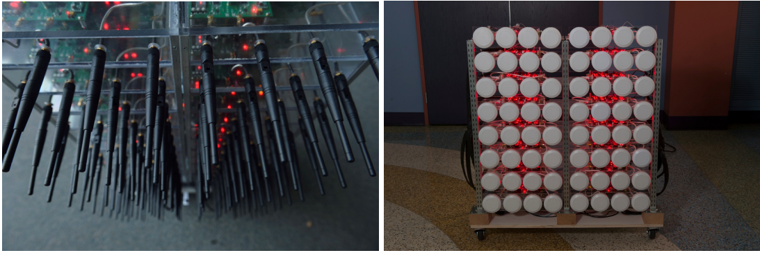
Figure 1.2: Massive MIMO APs from Rice Argos project [1] with many antennas.
