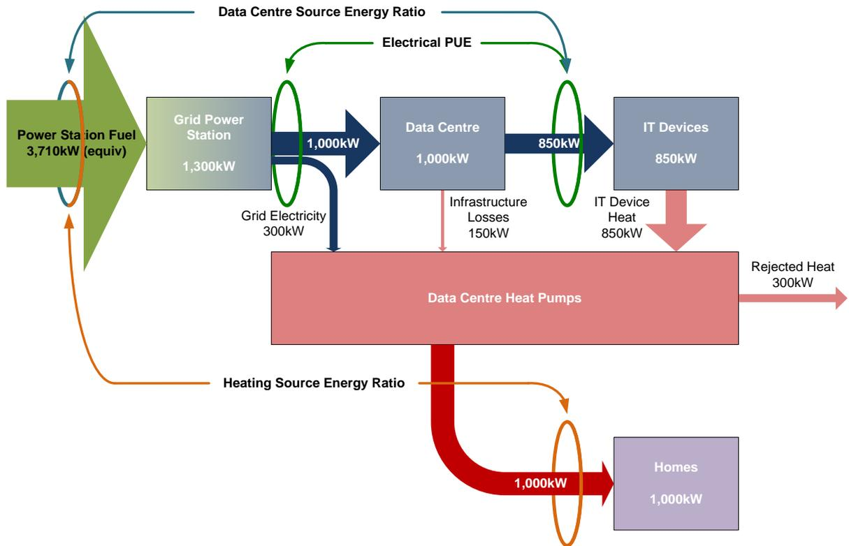
Figure 6 Cases B,C,D - PUE and Source Energy Ratio
