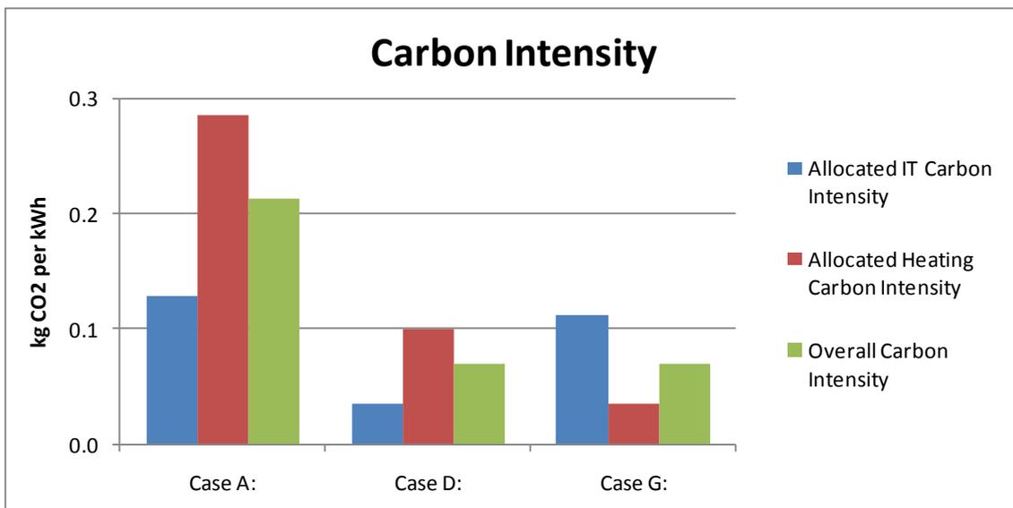
Figure 25 France carbon intensity - re-use has an SER of one
