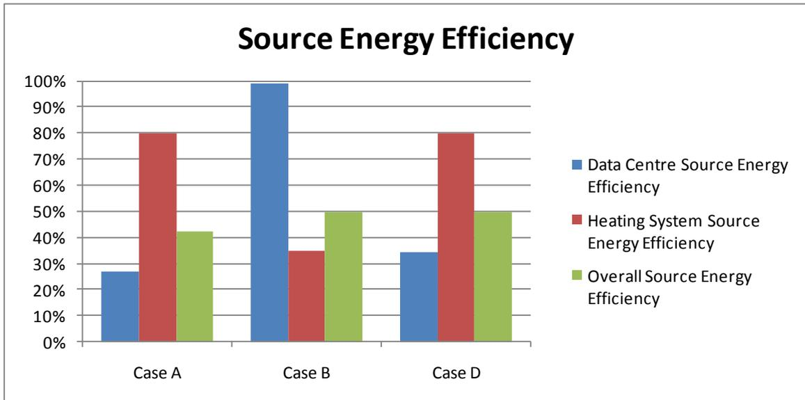
Figure 11 Annual Source Energy Efficiency Cases A, B and D
