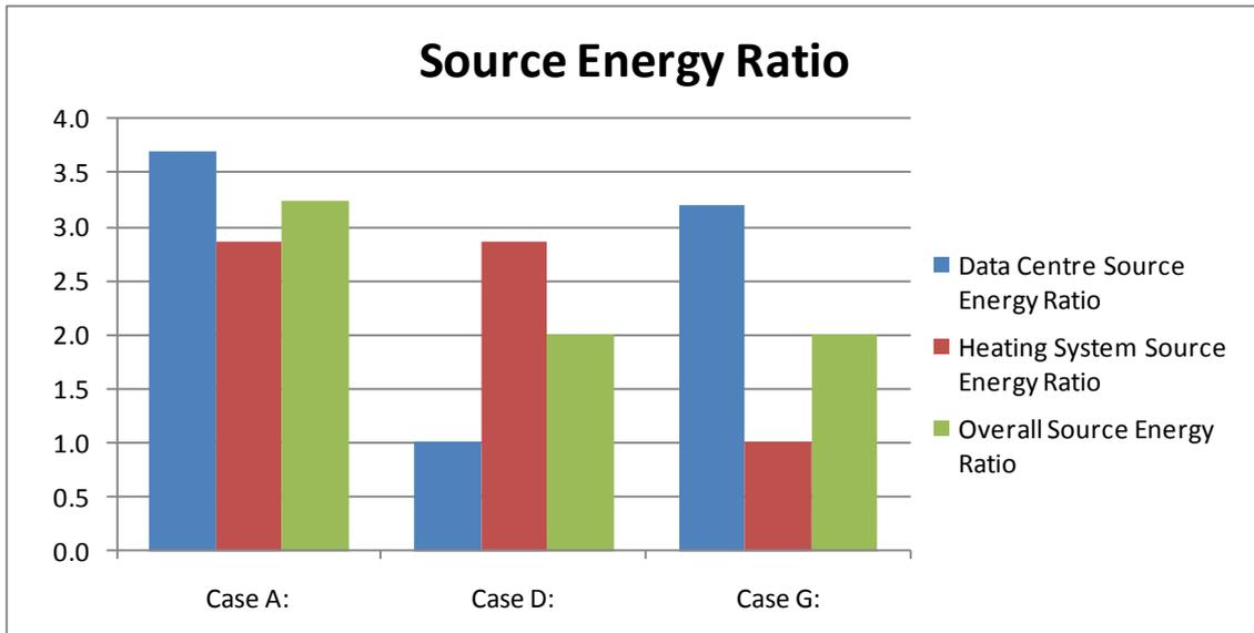
Figure 24 France Source energy ratio - re-use has an SER of one
