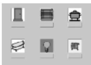
Figure 2 Screenshot of the visual Interface prototype representing six household appliances and their current status (i.e. door closed, blinds down, etc.).
