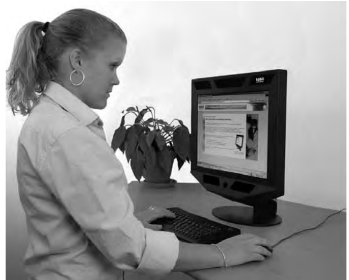
Figure 1 The Tobii 1750 remote eye-tracker.
