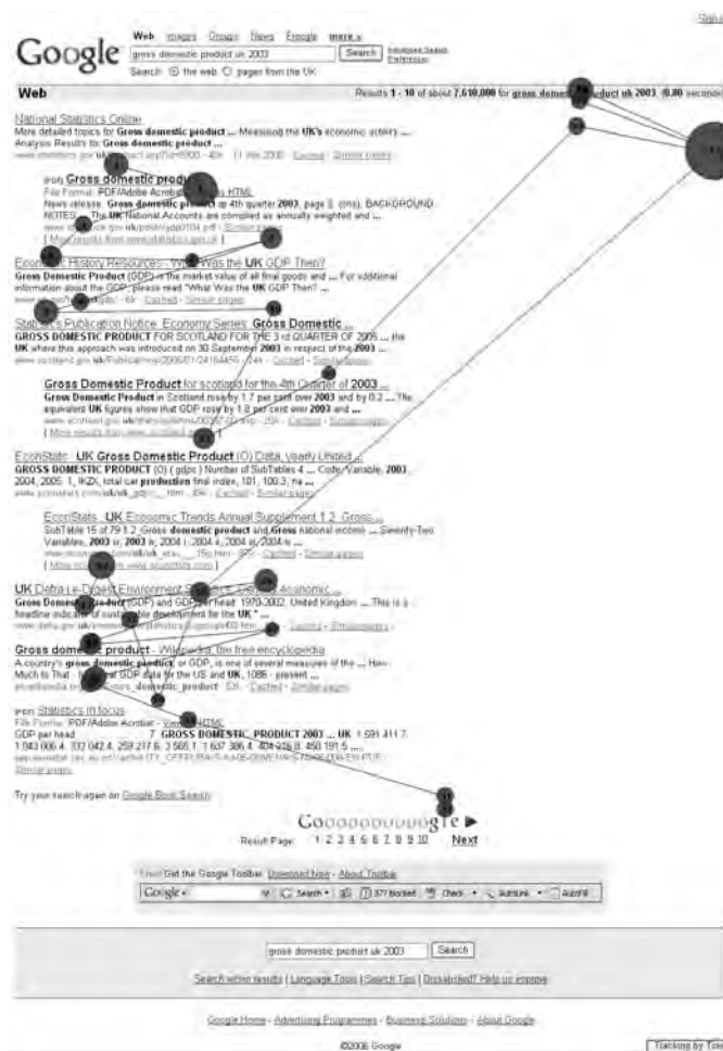
Figure 2 ClearView eye-gaze data replay. Dots represent fixation points that increase in diameter relative to fixation duration. Lines indicate the eye-movement scanpath.
