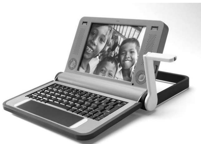
Figure 2 A prototype of the $100 laptop; this version is powered with a hand crank (right).
