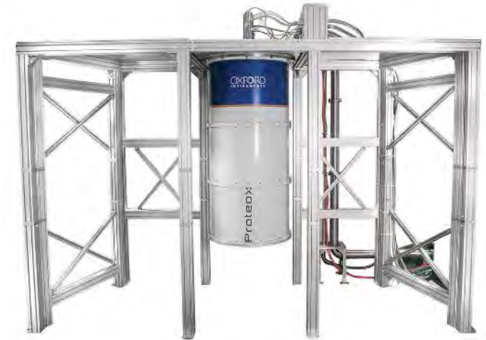
Oxford Instruments: ProteoxLX dilution refrigerator (Base temperature as low as 7mK)
