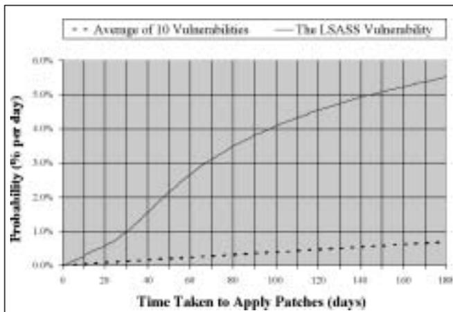
**Fig. 3. The probability of a successful worm attack**
