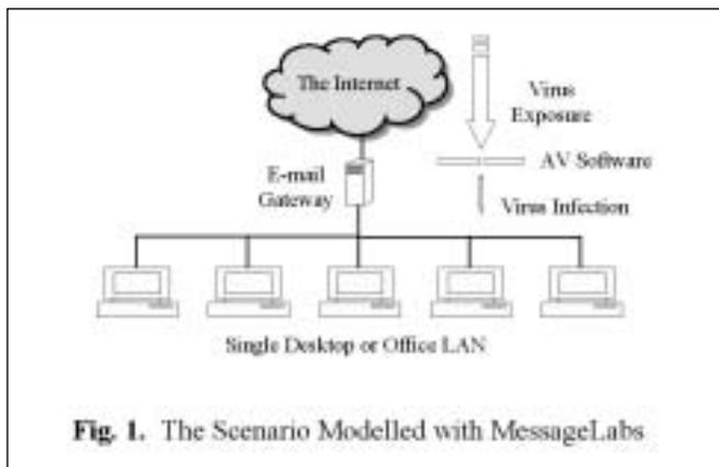
Fig. 1. The Scenario Modelled with MessageLabs
