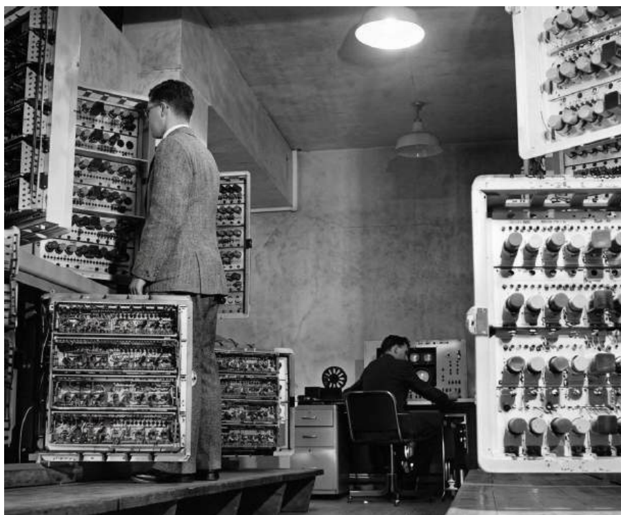
Figure 2: Photograph of the Manchester Ferranti computer with open racks from a 1953 publication.
