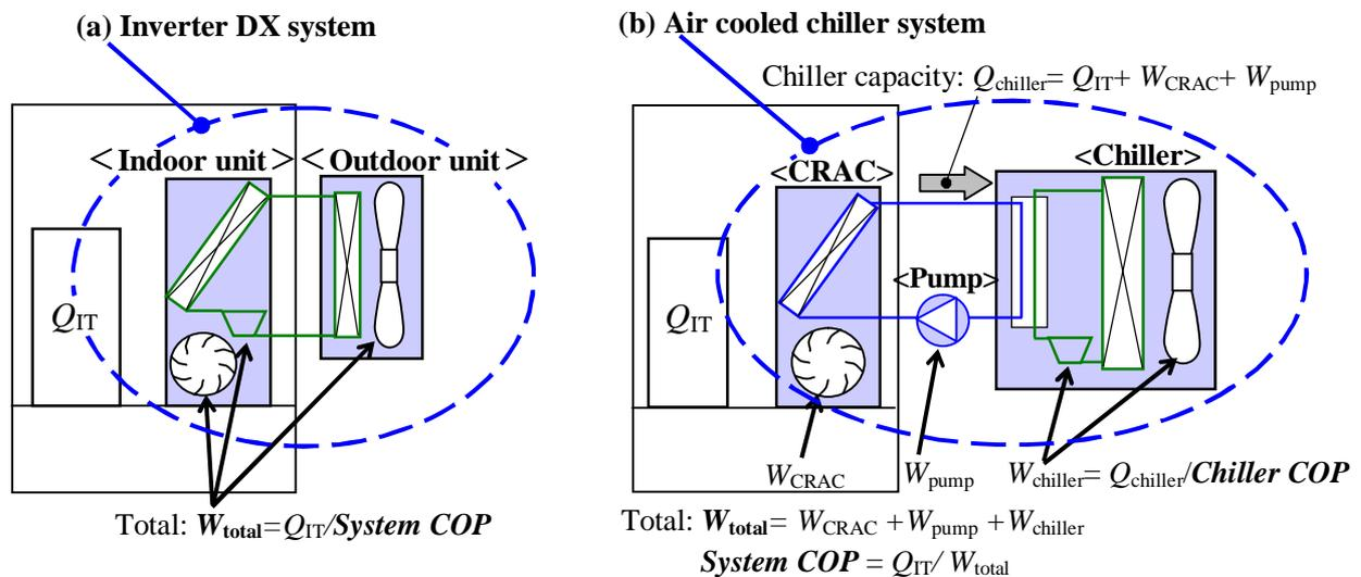
**Fig 2. Electric power consumption**
