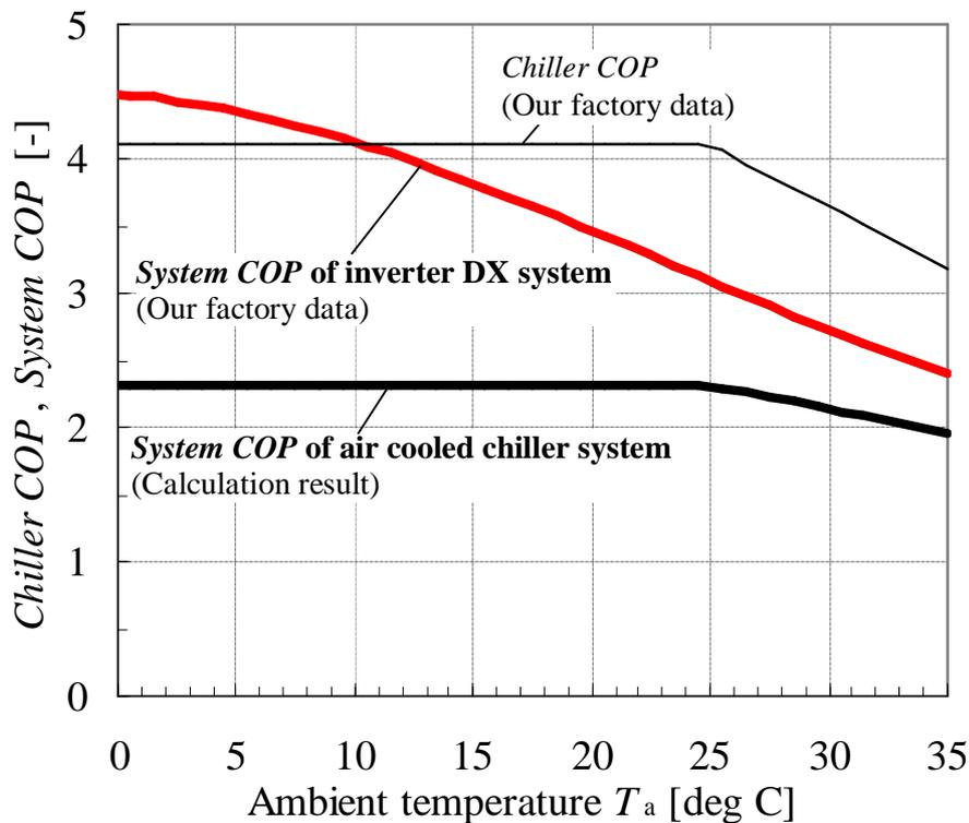
**Fig.4 Chiller COP and System COP for each ambient temperature**
