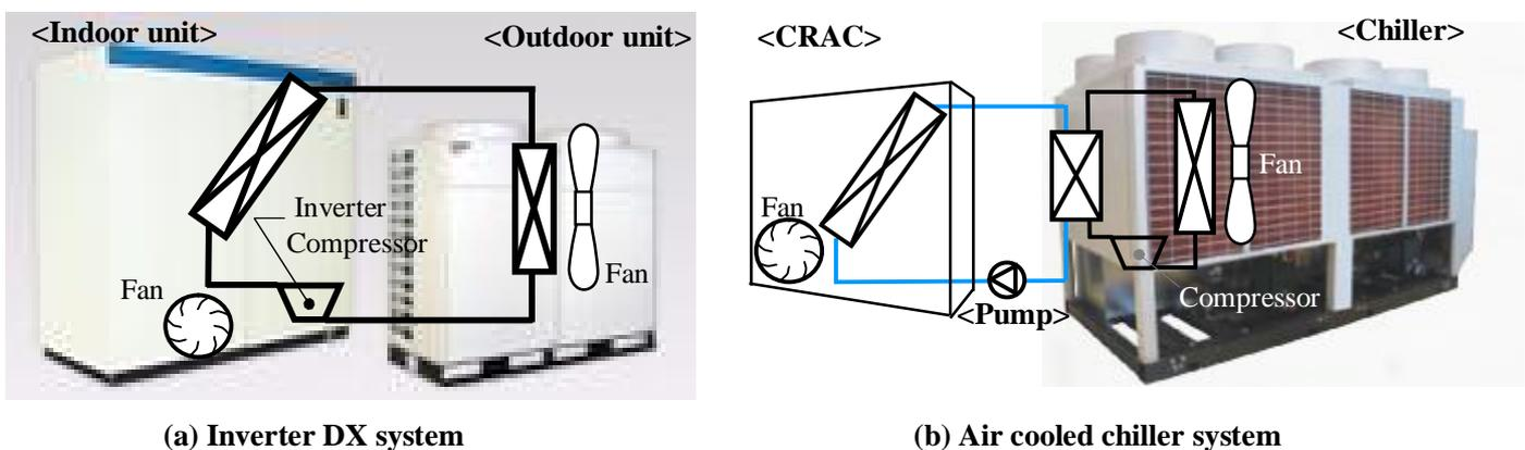
**Fig.1 System configuration**
