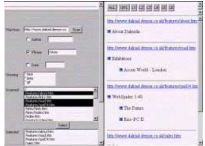
Webtree screen shot (running in a standard web browser, which is not shown). Queries are entered in the left frame, the right frame shows search results within an interactive outline.
